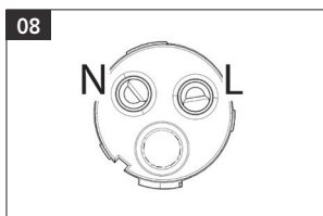
Connect the cables correctly to the core..
